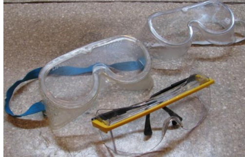
Fig. 1.1: Safety glasses. Use versions with ANSI Z87 label. ANSI is short for American National Standards Institute. Chemistry goggles, as also shown here, are not recommended for metal work, since they may block the vision too much.
