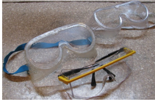
Fig. 1: Safety glasses. Use versions with ANSI Z87 label. ASNI is short for American National Standards Institute. Chemistry goggles, as also shown here, are not recommended for metal work, since they may block the vision too much.
