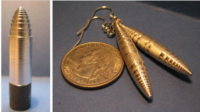
Fig. 15: Left) Cigar shapes made from a small diameter, O.D. 0.5", Al round using a manual benchtop lathe. Here turning cuts are used. Right) This also looks good as an earring when scaling it down.
