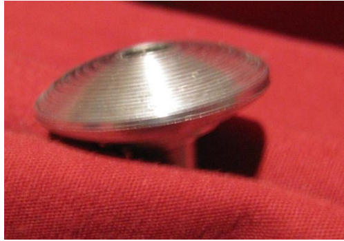
Fig. 13: "Cutting a UFO" as a facing operation. An O.D. 1" Al round was used. The work piece was drilled and tapped ( \frac{1}{4} "-20 screw), in order to cut an elliptical shape in both sides using a \frac{1}{4} " bolt. That piece has about the size of a US quarter and just landed.
