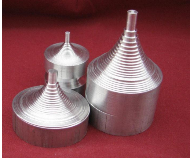
Fig. 9: Examples of spherical shapes made by slicing the metal rod using a manual lathe from Sherline. Ball ends can also be made.
