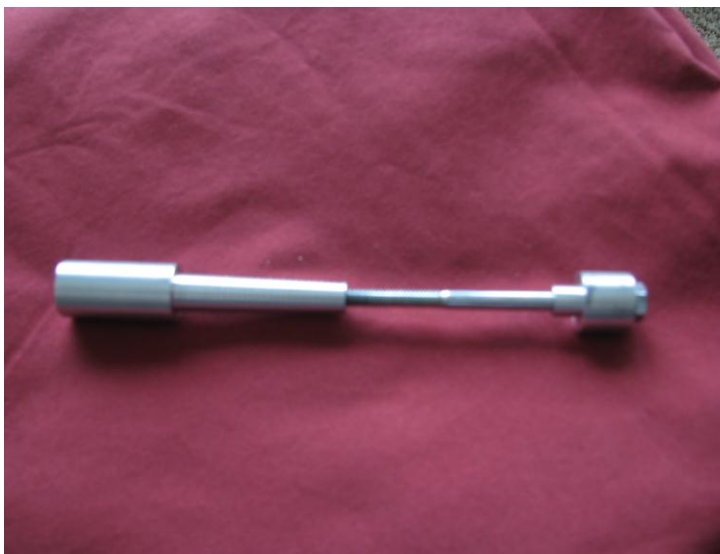
Project examples – special shapes made easily: Morse taper cut easily and precisely by slicing – engineering project
