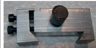
Dovetail lathe stop / mill lock
