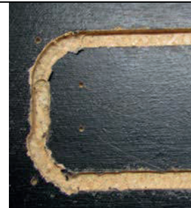
Keyways with rounded corners – flanges
