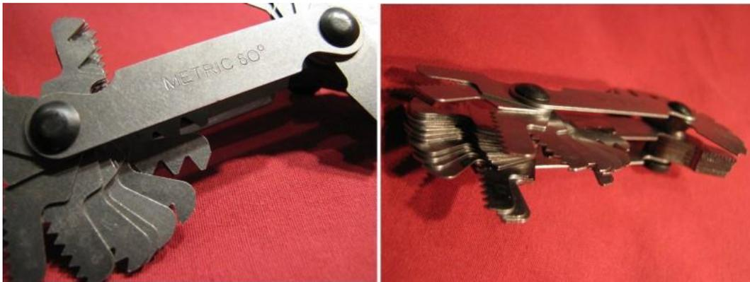
**Fig. 2.4a:** Metric / English combination thread gauge. (I doubt that you will ever need this. If you find a cheap one, perhaps, go for it. I got this one for a few dollars at Max shop.)
