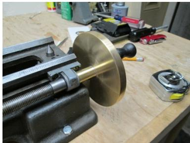
Now were off to making things, like a new handle for the lead screw. 4" diameter solid brass sure makes it easier to turn by hand. Along with purchasing a new tool post, some cutting tools, new brass gibbs for the tool post slide and compound swivel base.
