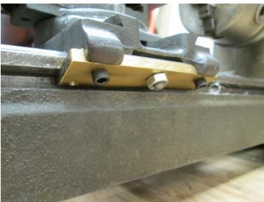
First thing was to make a new rear gib for the compound because mine was broken and it wasn't really a good design. New one made out of brass instead of the cast iron one that is stock. Also drilled and tapped it for 2 new screws to secure the Gib on both ends instead of the stock one in the center position.
