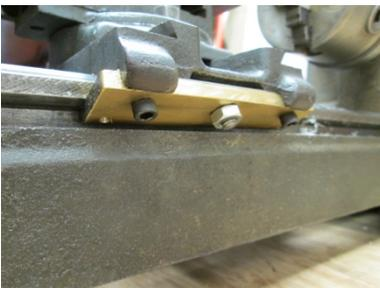
First thing was to make a new rear gib for the compound because mine was broken and it wasn't really a good design. New one made out of brass instead of the cast iron one that is stock. Also drilled and tapped it for 2 new screws to secure the Gib on both ends instead of the stock one in the center position.
