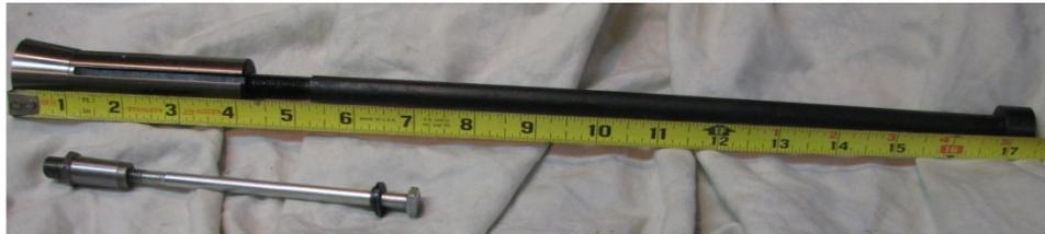
**Fig.:** Grizzly's drawbar with R8 collet also shown is Sherlines Morse taper for the headstock and the drawbar for it
