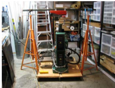
Fig. 26.4: Lifting the mill with low budget equipment from Harbor Freight Tools. Don't copy this, the risk is yours. High stand jacks tip over easily, to my experience
