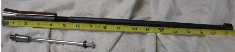
Fig. 26.3: Grizzly's drawbar with R8 collet, also shown is Sherlines Morse taper for the headstock and the drawbar for it
