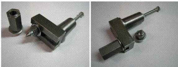
**Typical application:** Accessory for benchtop / tabletop lathes. Adapter mounts in a Morse arbor, e.g., in the tailstock spindle of a tabletop lathe and connects to a dead center (pin) or MT0 arbor.
