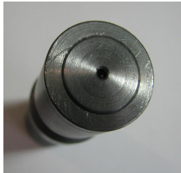
Buddy bar in a Morse test arbor. We see the small diameter end in this photo.
