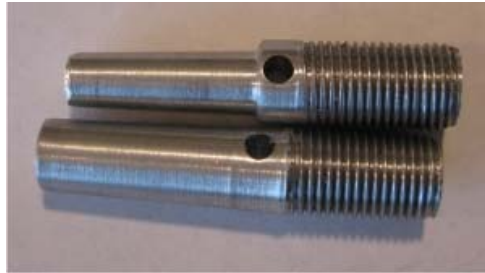
Fig. M10 – project example Morse #1 and Morse #0 to Jacobs chuck ( \frac{1}{2} "-20) adapters. Morse #0 to \frac{1}{2} "-20 is quite uncommon and hard to find. You can now make whatever size you need. Use a hex bar if you want to use a wrench. (Morse Tapers were cut with help of the LASER Protractor.)
