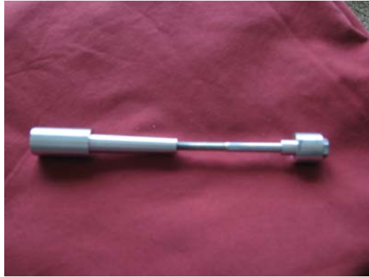
Fig. M4 – project example: Endmill holder. Perhaps the best way to perfectly center an endmill is to use a Morse type holder and drawbar, as shown here. (Morse #1 Taper was cut with help of the LASER Protractor.)
