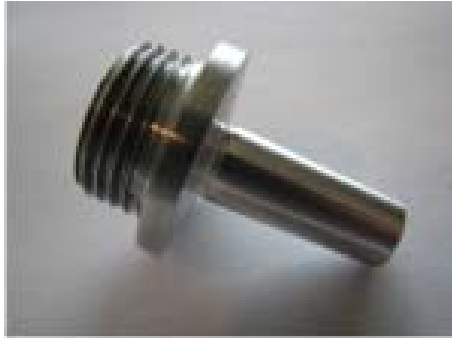
Fig. M7 – project example: Morse #0 to \frac{3}{4} "-16. Allows mount of a lathe chuck into the tailstock for, e.g., headstock drilling. A piece like that sells for around $40. (Morse #0 Taper was cut with help of the LASER Protractor.)
