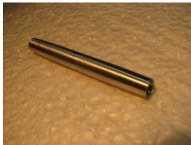
Fig. M6 – project example: Center with a concave end. This is sometimes useful when modifying a work piece with a pin end. (Morse #0 Taper was cut with help of the LASER Protractor.)
