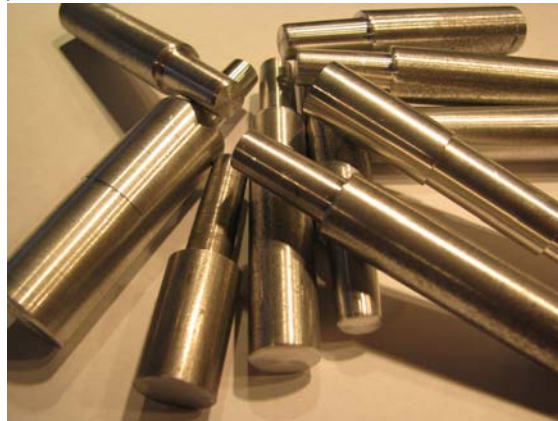
Fig. M8 – project example: You can now make Morse taper by the dozen – easily. Morse blanks in different sizes and different materials. (Morse #0 Taper was cut with help of the LASER Protractor.)
