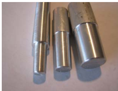
Fig. M9 – project example: Left to right Morse #0, #1, and #2 blanks. Although a #2 Morse taper is more common on full size systems, it is actually simpler cutting it precisely on a small lathe. (Morse Tapers were cut with help of the LASER Protractor.)
