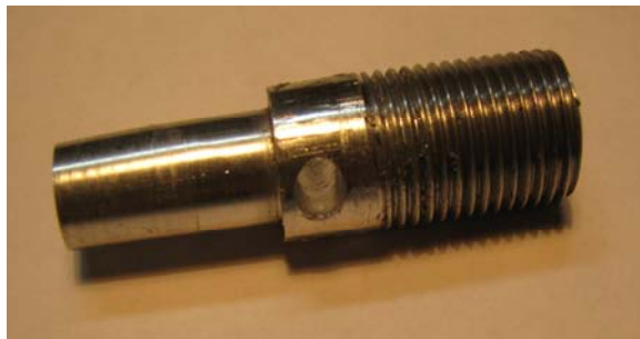
Fig. M3 – project example: Jacobs chuck (1/2-20) to tailstock Morse #0 adapter. Less expensive Jacobs chucks, including larger sizes, are often available. However, typically they come with a tapered hole and not with a Morse #0 taper. (Morse #1 are easily commercially available, but Morse #0 ...) This type of an adapter is shown here: $1 for materials, 20 min work. (Morse #0 Taper was cut with the help of the LASER Protractor.)
