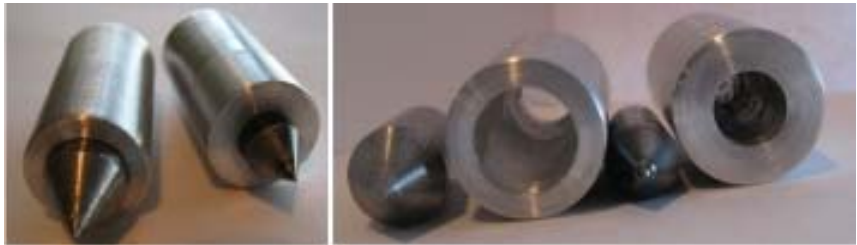
Fig. M11 – project example Morse #1 and Morse #0 arbors. (Internal Morse tapers were cut with help of the LASER Protractor.)
