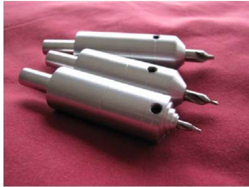
Fig. M2 - project example: inexpensive chucks for center drills. A good Jacobs drill chuck with Morse adapter would cost you probably close to $50. (Morse #0 Tapers were cut utilizing the LASER Protractor.)
