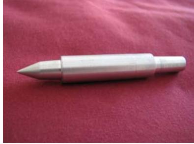
Fig. M1 - project example: cutting a perfect Morse taper. Extended tailstock center. (Morse #0 Taper cut with the help of the LASER Protractor.)
