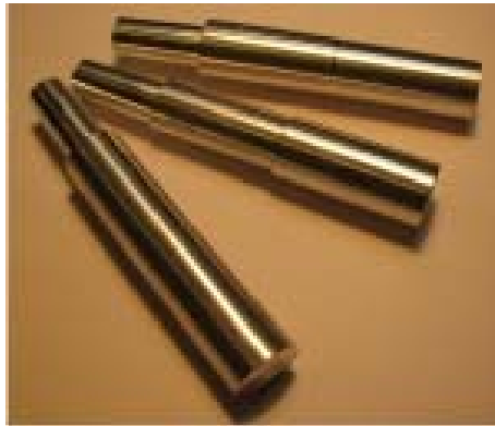
Fig. M5 – project example: Morse #0 blank adapters are the starting point for most tailstock tools. These shown here have O.D. \frac{1}{2} " and are 3" long. However, you can now make whatever size you may need. These typically cost $7-$20/piece. (Morse #0 Taper was cut with help of the LASER Protractor.)
