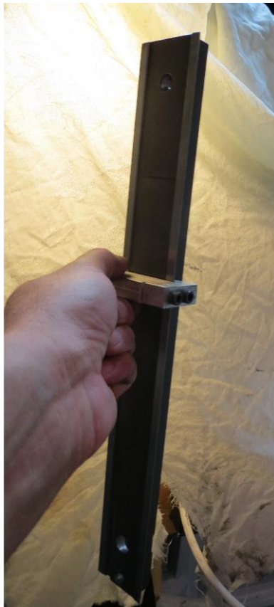
Fig.: How well does the dovetail clamp on the lathe bed? See by yourself. You can hand up a Sherline lathe bed in your shop using our dovetails. We test accessories on more than one Sherline system, of course. Making sure that variations in the production don't affect our accessories.
