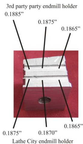
This figure shows a test of endmill holders. A 3/16 in. (0.1875 in.) endmill was used. The width of the keyway was indicated.
