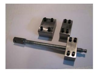
The design The all steel vise (e.g. Sherline's vises are cut from aluminum) is a so-called plane mill vise. It consists of three brackets. Two are stationary and directly screwed on the mill table using steel T-bolts. One acts as a jaw the other holds the lead screw. The third bracket (or jaw) moves along the mill table by
