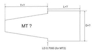
**Typical application:** Accessory for benchtop / tabletop lathes. Adapter mounts in a Morse arbor, e.g., in the tailstock spindle of a tabletop lathe. Perhaps someone recognized that more time is lost clamping center drills and drill bits in Jacobs drill chucks than is necessary. These simple, affordable, and useful accessories give one a fast tool-change system.
