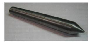
Morse taper – extended dead center. This accessory has a Morse taper at one end and a ~30° pin (taper) at the other end. The steel pieces can be used as a dead center. The length of the center can be customized. These pieces are cut from (non-hardened) steel, but the pin end will wear out over time (as usual, use cutting oil when using dead centers). However, any (hobby) machinist can easily resharpen the pin end. We also offer versions which have a tool steel pin inserted.
