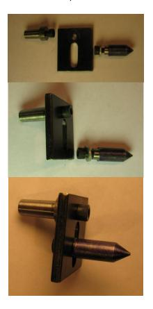
Assembling the tool. To save on shipping costs, this tool is shipped disassembled. For mounting it, two screws need to be tightened, see images.
