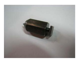
Size and details The bearings we use have an outer diameter (O.D.) of only 5/16" and an inner shaft diameter of 1/8". A  $\frac{1}{4}$ " O.D. tool steel pin (60° included angle) is pressed in the bearings. The bearing is pressed in a hex shaped steel arbor that is
